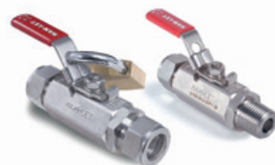
Ball Valves with Locking Device H-700 series MAWP: 2000Psi (137 bar) MAWT: 400°F (204°C)
