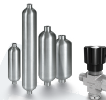
Ham-Let Sample Cylinder and Needle Valve with Rupture Disc MAWP: 3,000psi (206Bar) MAWT: -58F to 450F (-50C to 232C)
