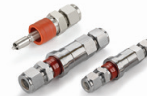
QCLOK® Quick Connectors 1/4", 3/8", 1/2" MAWP: 3000Psi (413 bar) MAWT: 500°F (260°C)
