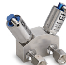
Multi Port Monoblock Valve HMB MAWP: Up to 150 Psi MAWT: -10 to 60°C
