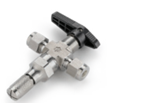
Metering Ball Valves MBV series MAWP: 2000Psi (137 bar) MAWT: 300°F (150°C)
