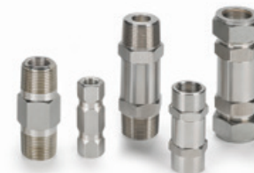
Check Valves - High Pressure, One Piece & Adjustable H-400 series MAWP: 6000Psi (413 bar) MAWT: -40° to 250°F (-40° to 121°C)
