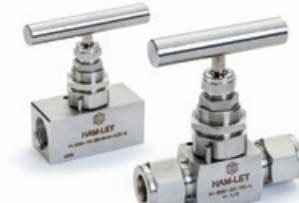
High Pressure Needle Valves H-300U series MAWP: 10,000Psi (690 bar) MAWT: 1200°F (648°C)
